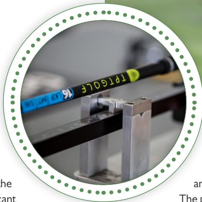
When making a tube from composites, the layer of material being wound or rolled into the tube has a start and an end. If the wall thickness is, for example, 2mm and the building material is 0.3mm, as typically used in the composite industry, then the start and end of the material in the tube wall can have a significant and unbalancing effect resulting in fibre misalignment and a spine that spirals along the tube.
