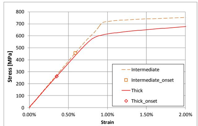
Fig. 6: Simulated stress-strain curve for the thick (300 g/m<sup>2</sup>, n=1) and intermediate-ply thickness (100 g/m<sup>2</sup>, n=3) quasi isotropic unnotched tensile test.
