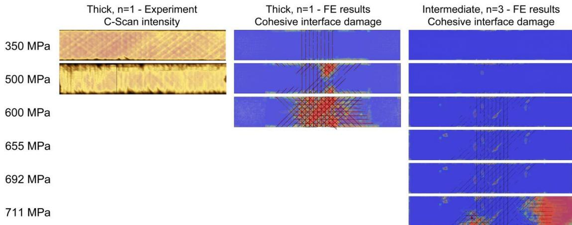
Fig. 7: measured and simulated cohesive element damage progression showing clearly the propagation of transverse cracks and delamination initiated at the free edges of the specimen.
