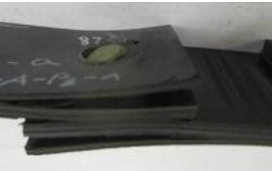
Thick ply specimen after bearing strength test
