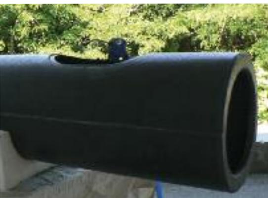
Picture of the outer skin preform after draping in the lower mold for tail boom
