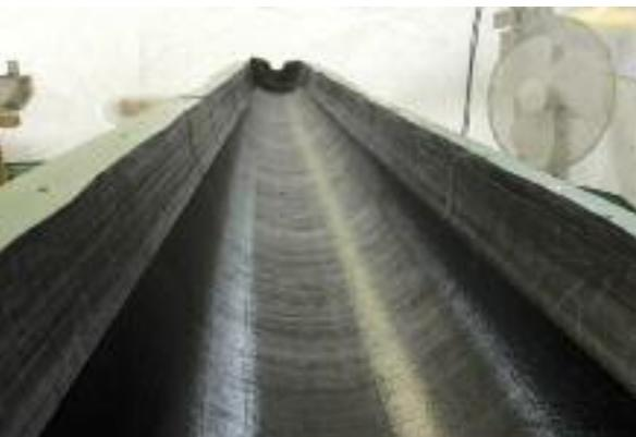
Once the pre-form was given final trim and sent to BHR in Anglet, France, it was impressively fast and easy for BHR's lamination team – assisted by a representative from the TPT® team - to place the pre-forms and the sandwich core in the tail boom mold, even for this first component produced. BHR's management team was able to assess the potential of the Thin Ply Technology on the basis of this initial experience and is planning to implement the technology at the industrial production scale.
