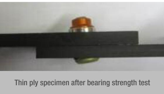
Thin ply specimen after bearing strength test
