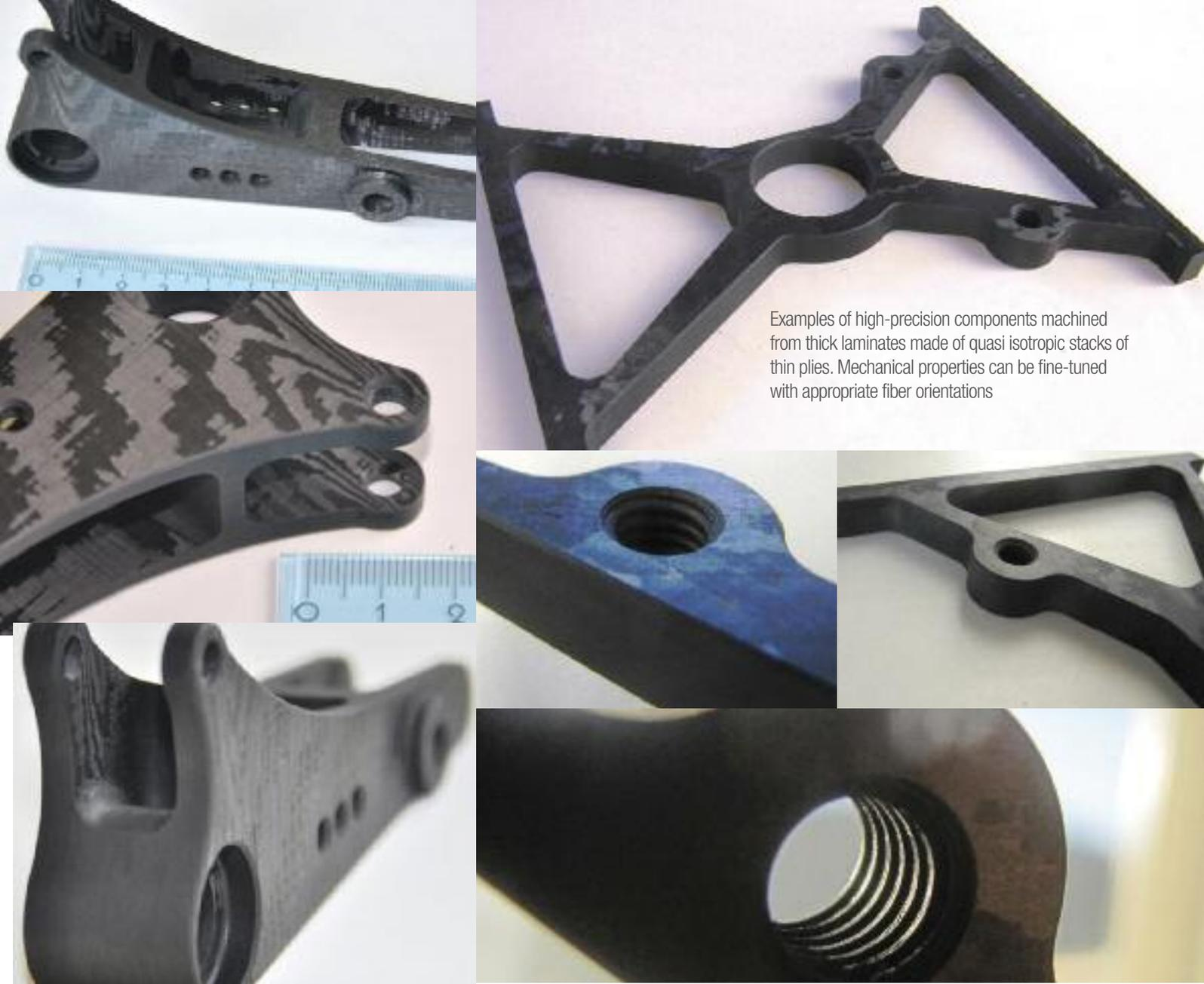
Examples of high-precision components machined from thick laminates made of quasi isotropic stacks of thin plies. Mechanical properties can be fine-tuned with appropriate fiber orientations
