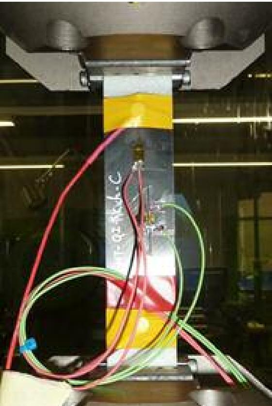
Quasi isotropic tensile test specimen equipped with acoustic emission sensors
