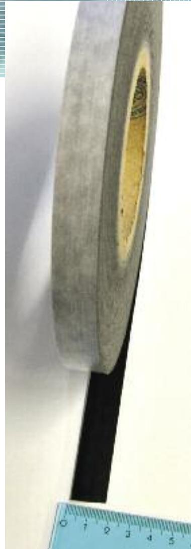
Example of slit prepreg roll, width: 16mm
